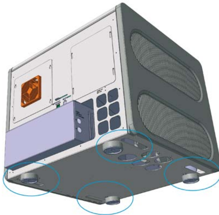
Figure 3 Diagram showing the location of carrier grips at the instrument base plate.
