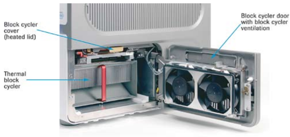
Figure 11 Block cycler door opened allowing a view of the inserted thermal block cycler and block cycler cover
